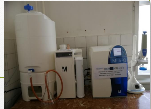
Device for preparing redest. water
